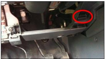
The ECU communicates using the CAN Bus on the OBDII connector. Connector pinout as well as connection table are shown here below
