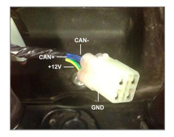
Here below you see the bike connector pinout and the connection table.
