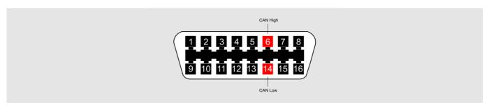
OBDII connector pin Pin function AiM cable
