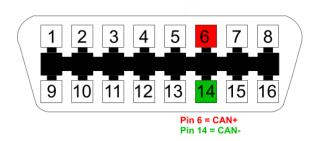
To connect AIM logger with the OBDII connector (shown here above on the right):
