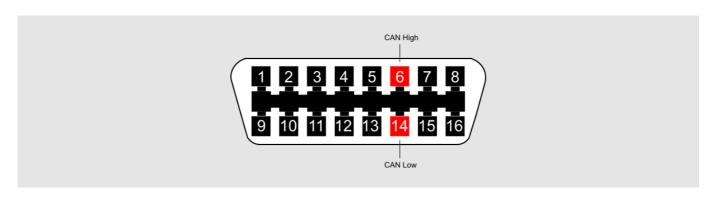
OBDII connector pin Pin function AiM cable
