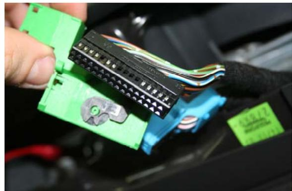
To connect AIM logger to Bosch 7.8.1. ECU:
