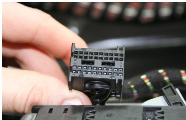
To connect AIM logger to Bosch 7.8.1. ECU connector, please connect cable labelled CAN+ of the logger with the light blue/white cable (pin 36) – of the ECU connector, and cable labelled CAN - with the grey/white (pin 37) cable of the ECU connector.
