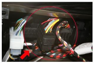
To connect AIM Logger to service connector, please connect cable labelled CAN+ of the logger with yellow/white cable (pin 28) of the service connector and cable labelled CAN-with black/white(pin 29) cable of the ECU connector.
