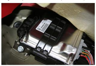
To connect AIM logger to Siemens EMS SDI 3.1 ECU connectors, please connect cable labelled CAN+ of the logger with the yellow/white cable (pin 54 – A connector) – of the ECU connector, and cable labelled CAN - with the black/white (pin 41 – A connector) cable of the ECU connector.
