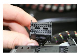
To connect AIM logger to Bosch 7.8.1. ECU connector, please connect cable labelled CAN+ of the logger with the yellow/white cable (pin 36) – of the ECU connector, and cable labelled CAN - with the black/white (pin 37) cable of the ECU connector.
