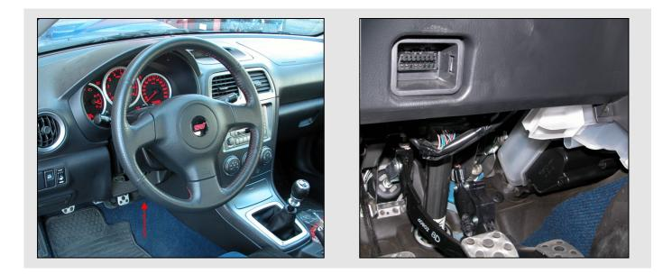
The ECU communicates using the CAN Bus on the OBDII connector. Connector pinout as well as connection table are shown here below.
