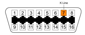
OBDII connector pin Pin function AiM cable
