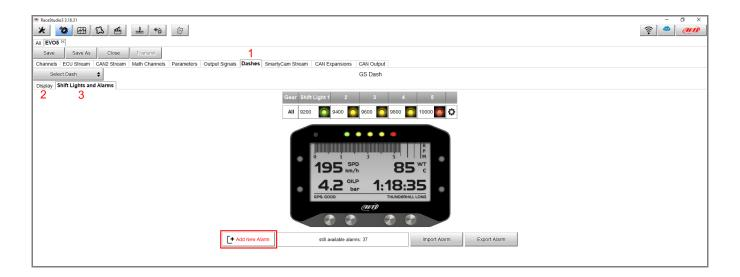
• in the Shift Lights and Alarms add new alarm, after a name has been assigned and the conditions have been set, using the desired channels (add/remove more conditions clicking the drop-down menu it is possible to choose the associated action type
