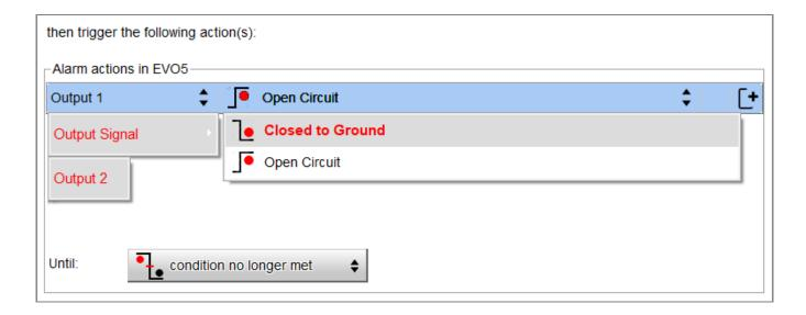
This function can also be accessed from the Output Signals tab of Race Studio 3: this is mainly used when no dash is connected to EVOx.
